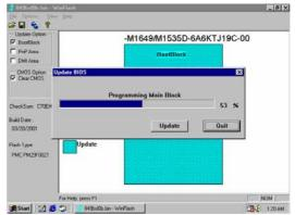
When System programming BIOS don't turn off power after finish update BIOS, the system will clear CMOS and automatically Restart
